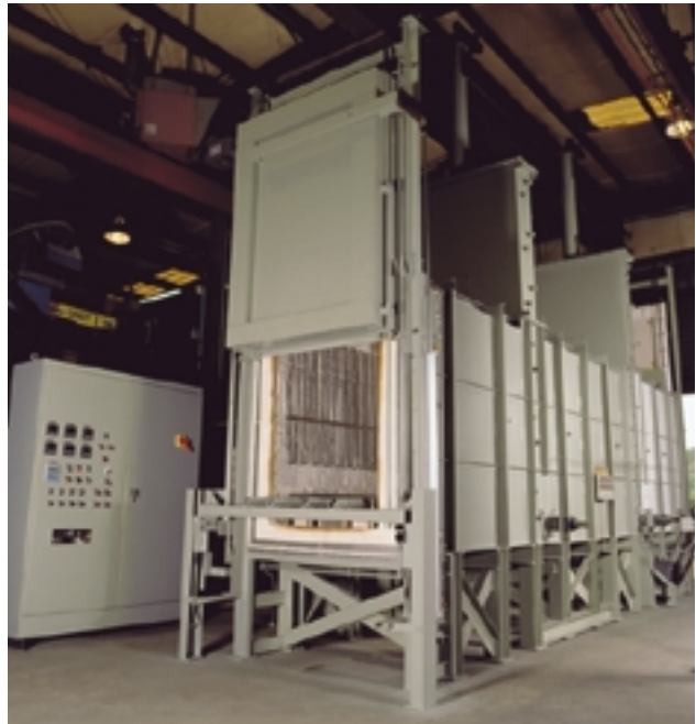
This is a special furnace designed for continuous ferritic carbonitriding.
